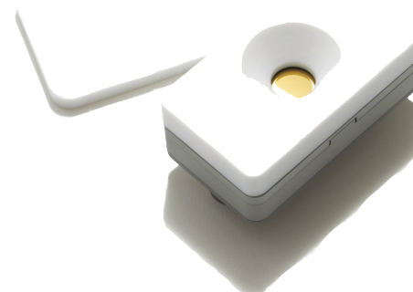
FIGURE 1. The Q-Sense Open module is suited for pipetting directly onto the sensor surface.
